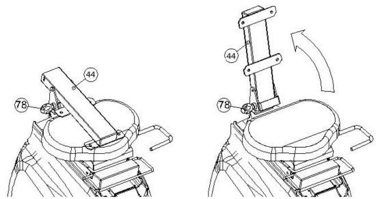
Hold Knob (78) and pull to release the Back Cushion Support (44). Place it in an upright position. Make sure the Knob (78) is then fixed firmly back in place to secure the Back Cushion Support (44).
