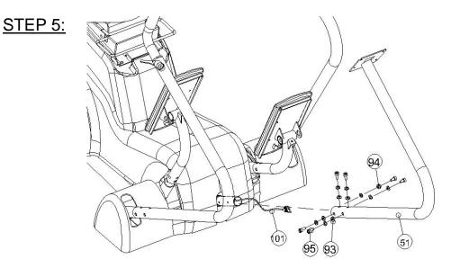
Taking Control Wire (101) feed it through the Computer Post (51). Next, attach the Computer Post (51) to Main Frame (2) using the Curved Washer Ø6.2\*Ø13\*1T (93), Spring Washer SW6(94) and Hexagonal Bolt M6\*10L (95). Make sure the bolts are securely tightened.
