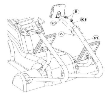
Remove Bolts M5\*10L(A) from the back of the Computer (96). Connect Control Wire Computer (B) to the Control Wire (101). Then using Bolt M5\*10L(A) attach the Computer (96) to Computer Post (51). Make sure the bolts are securely tightened.
