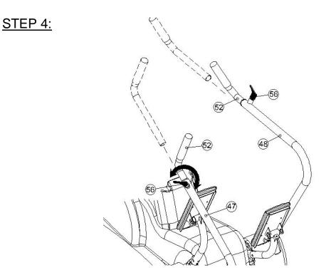
Release Knobs (56) and then insert Moving Handle Set (52) into Moving Handle R (47) and Moving Handle L (48). Tighten the screw Knob (56) according to user's preference. The Handles can be adjusted to various users' lengths.
