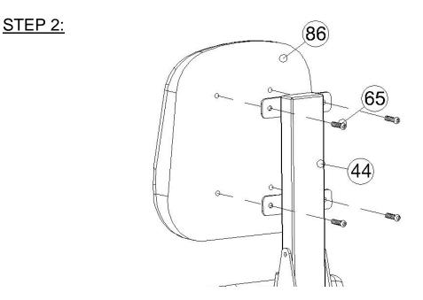
Assemble the Back Cushion (86) by using the Hexagonal Bold M8\*15L (65) to secure the Back Cushion Support (44). Make sure the bolts are securely tightened.
